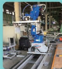
行走軸結合棧板堆疊系統 Robot Linear Axis combined with Paletizing
