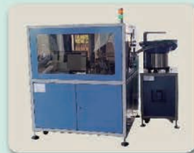
震動盤結合影像辨識 Image recognition system combined with Vibrator Bowl
